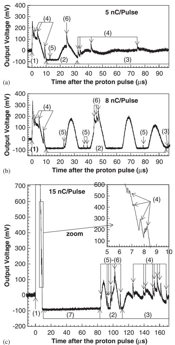
Fig. 1. Waveforms (output voltage as a function of time) recorded after one proton pulse with a  $^{235}\text{U}$  coated solar cell (without compensation) in the LSDS, for 3 different proton pulse sizes: 5 nC (a), 8 nC (b) and 15 nC (c). Time 0 corresponds to the incident proton pulse. Fission signals are indicated by arrows (see text for additional discussion).
