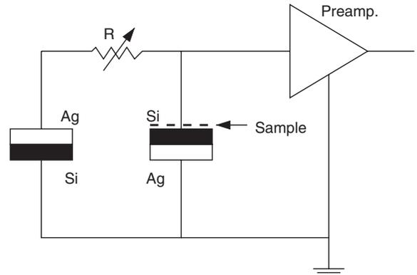
Fig. 5. Diagram of a refined compensation system. A potentiometer  $R$  is inserted between the two cells.
