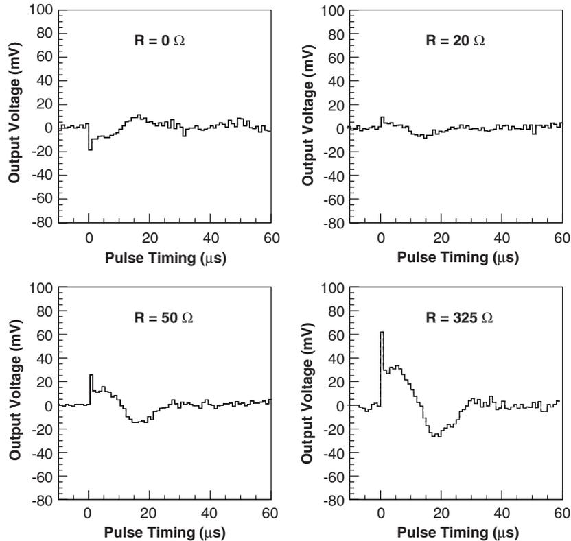
Fig. 6. Response of the compensated solar cell to the same  $\gamma$ -flash with four different values of the potentiometer. In order to perform a fine adjustment, the compensating cell had a slightly higher gain than the compensated cell. Therefore, the signal is negative for  $R = 0 \Omega$ .
