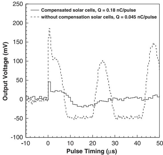
Fig. 3. Response to a  $\gamma$ -flash (at  $t = 0$ ) with (full line) and without (dashed line) compensation (identical cells, no fissionable material). Note that the electron beam intensity was larger by a factor of 4 in the case of compensated setup: 0.18 vs. 0.045 nC/pulse. Therefore, the compensation reduced the  $\gamma$ -flash peak by a factor of 20.
